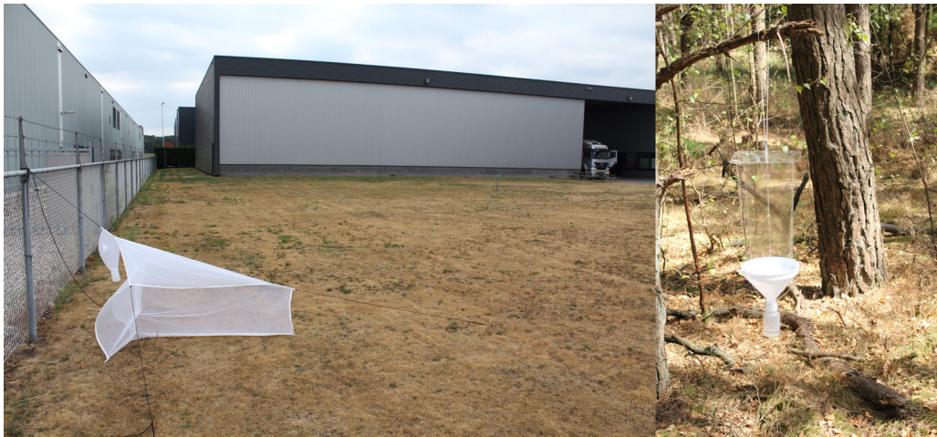
Figure 4.7. Townes model Malaise trap on the left, window trap on the right. Note these are examples of many Malaise and window trap models in use. Pictures by Bas Oteman.
